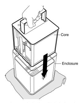
With a flat hand, press down on the latch until it locks into place. Firmly press the core to ensure it is fully secured within the enclosure. (Figure 21)
